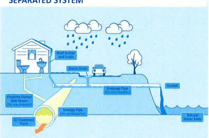
The picture shows the municipal separate storm sewer systems When you flush your toilet or run water down the drain, we have a separate sewage pipe for wastewater that goes to the treatment plant.
